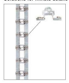
Single LEDs are clinched unto steel tracks using the TOX®-MICROpoint. The joining of steel and copper is easily accomplished and provides good dynamic retaining strength. The thermal connections done up to now on the electrical assemblies were problematic.
