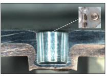
Cross section of a TOX®-MICROpoint on the LED strip. The strip is made up of galvanized steel 0.6 mm thick and galvanized copper 0.5 mm thick (point-Ø 2.0 mm). Even this miniature version of the TOX®-Round Point shows the typical interlocking of the clinching process.
