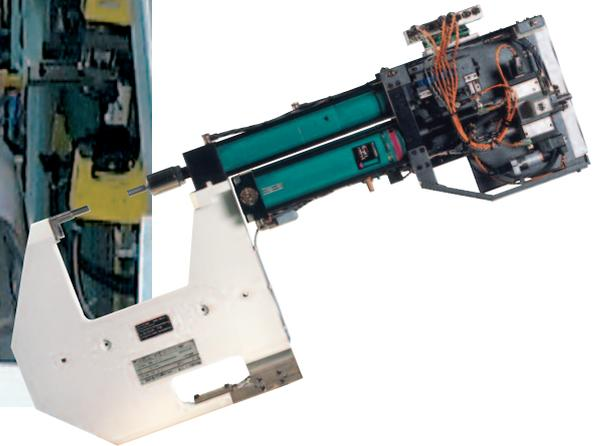
Application of 3 TOX®-Powerpackage cylinders in a series valve production. High frequencies, compactness and reliability over millions of cycles are the basis for satisfied customers.
