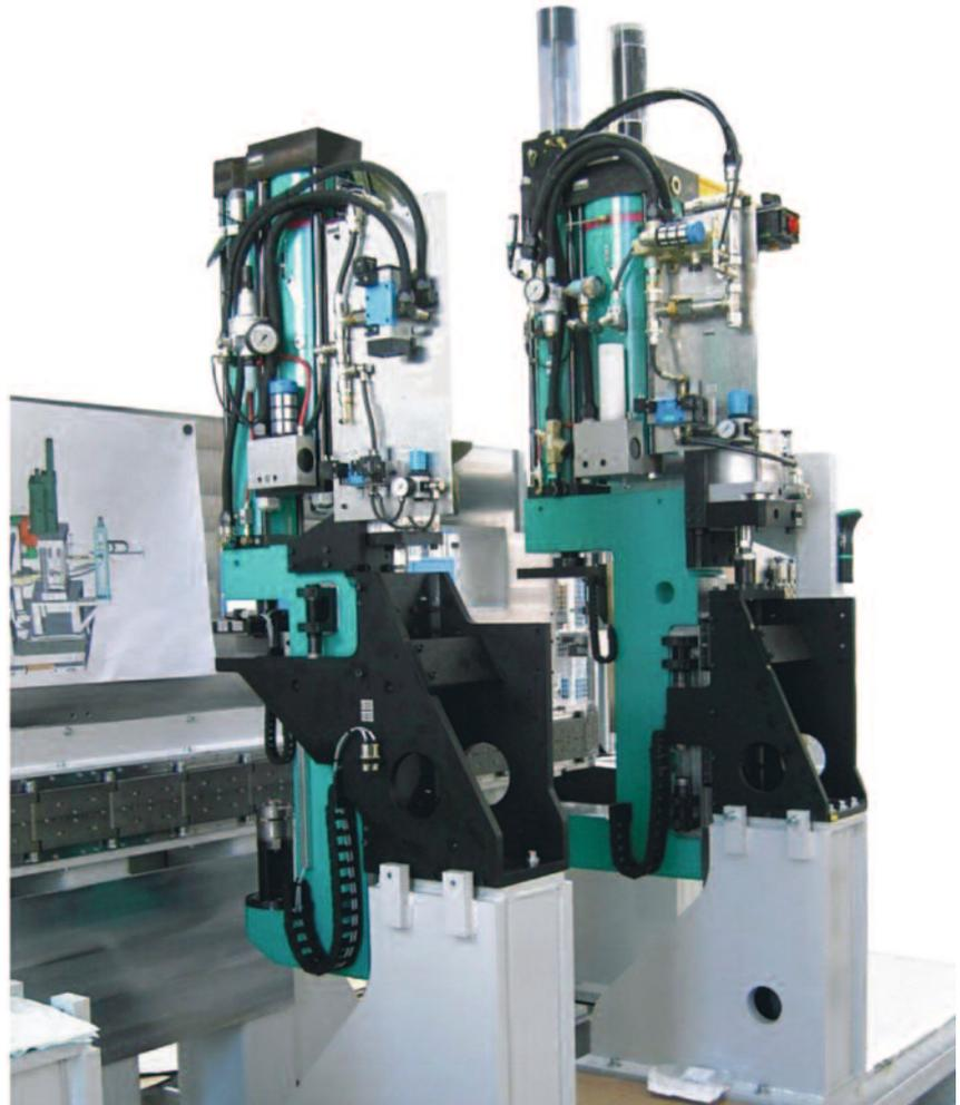
The TOX®-Powerpackage can be easily mounted on linear tracks, thereby providing a simple, flexible customized machine. Simplicity is further provided by the lack of hydraulics and the use of simple controls.
