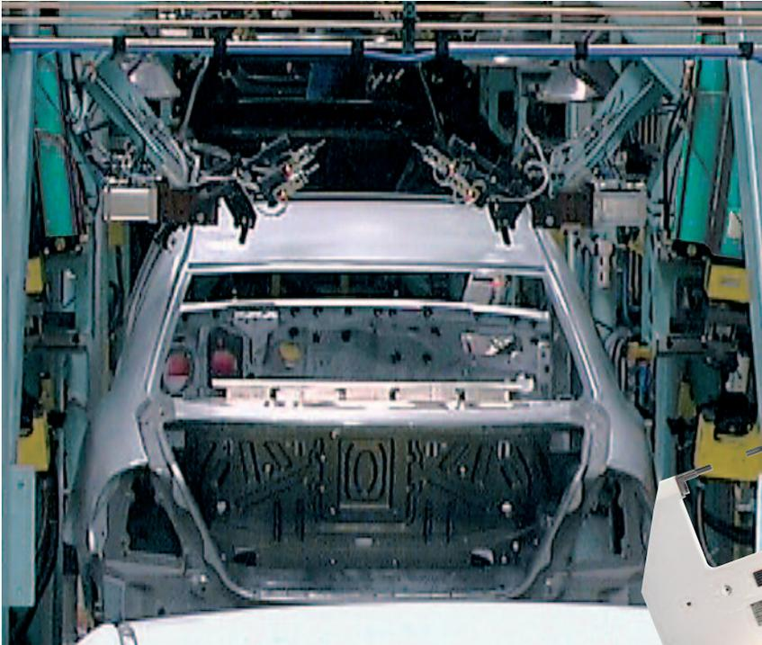
**TOX®-Robot Tongs and TOX®-Machine Mount Tongs**
