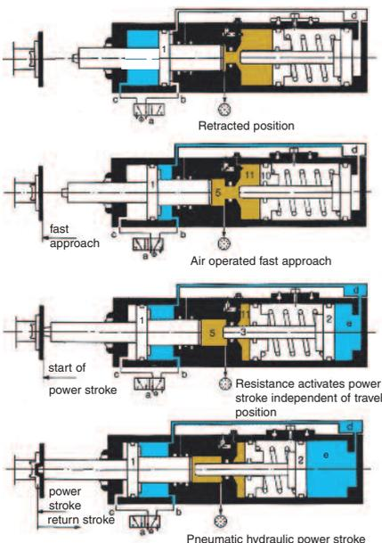
Fast approach - the main control valve "a" is switched. The working piston 1 extends at high speed until it meets resistance at any point of the stroke. This resistance causes the changeover of the included power stroke sequence valve "d".
