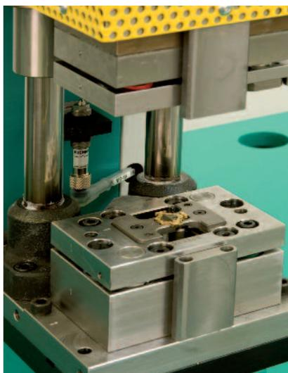
The metal rings are stamped directly from a sheet metal coil. They form the individual pieces for a contact tab of a mechanical switch prior to clinching. The pieces are loaded into a multipoint die set and are clinched together in one cycle with the TOX®-MICROpoint.
