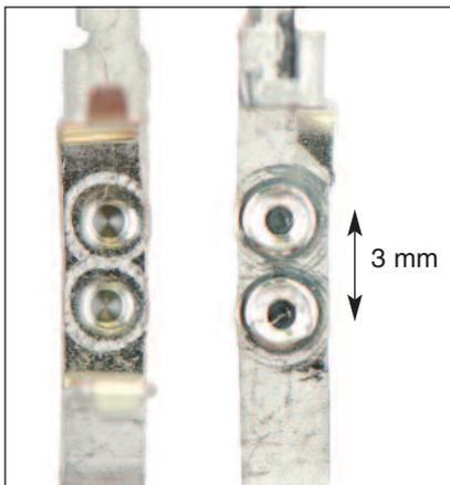
The picture on the left shows two TOX®-MICROpoint joints on a contact tab viewed from the punch side (cavity, left) and from the die side (protrusion, right). The carrier plate is not shown. The surface tin coating remains intact even inside the clinched point. This guarantees good conductivity.
