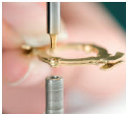
The actual cycle time for the TOX®-MICROpoint clinching process is **less than 0.5 seconds**, thus allowing cycles up to 150 strokes/min in eccentric- or special TOX®-Powerpackage-Presses.
