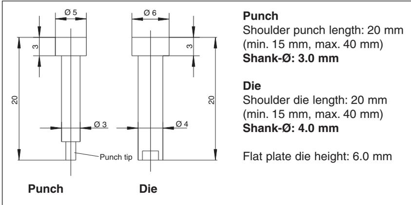
Mounting dimension tolerances are the same as our specifications in data sheet 80.100, which also contains an overview of our stripper systems and the multipoint capabilities of clinching.
