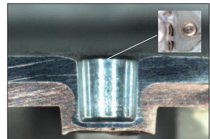
Cross section of a TOX®-MICROpoint on the LED strip. The strip is made up of galvanized steel 0.6 mm thick and galvanized copper 0.5 mm thick (point-Ø 2.0 mm). Even this miniature version of the TOX®-Round Point shows the typical interlocking of the clinching process.
