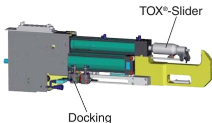
Robotic tongs with TOX®-ClinchRivet swage head and docking gate in loading position.
