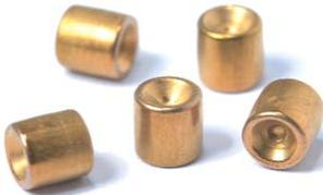
Sheet metal joining system with special die and full rivet for the permanent, perfect joining of metal plates (steel, aluminium etc.). A joining system similar to self-piercing-riveting but without cutting, i.e. the surface including the coating of the sheets to be joined remains intact like in the case of the TOX®-joint.
